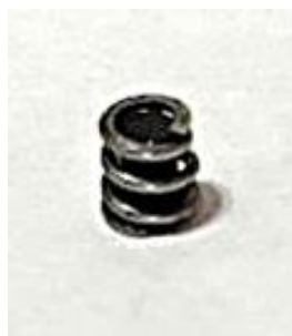
A well-used extractor spring and insert. Note they are the same height.
