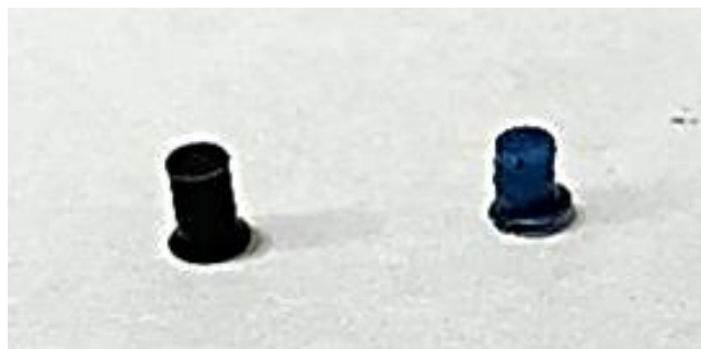
The modern nitrile black insert and the original silicone blue insert
